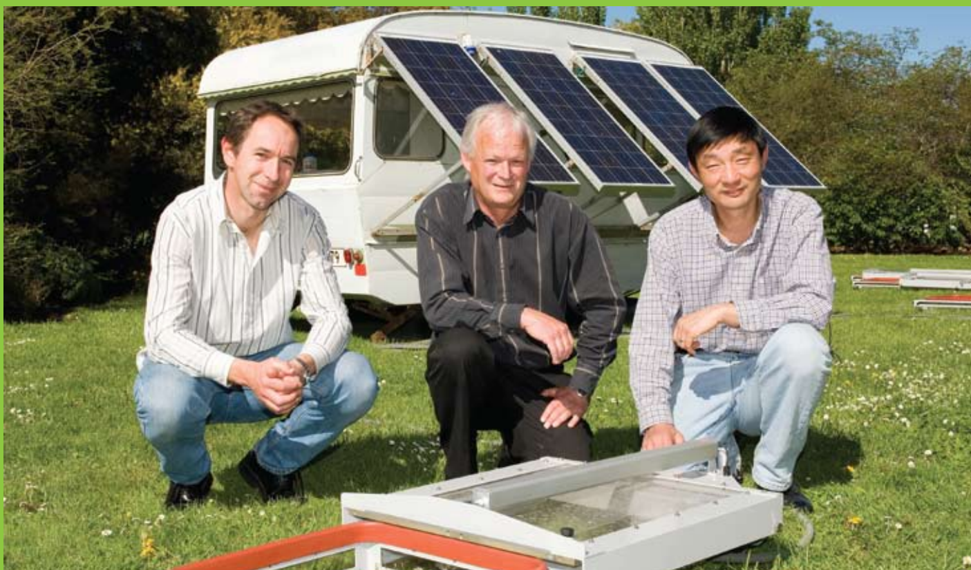
Soil Scientist Dr Tony van der Weerden (left), and engineers Steve Gebbie and Hong Zhang with the caravan-based system which automatically measures nitrous oxide emissions in fields.
